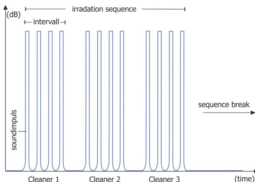
The number of acoustic cleaners (sonic horns) and sound wave sequences need to be adjusted to fit specific local conditions. The length of the sound impulse generally lies between 4 and 6 seconds. Normally, 4 impulses are delivered per sound interval. The sequence break varies from 10 minutes to several hours.
