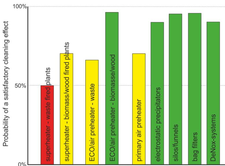
Since every type of facility works differently, it is impossible to guarantee a 100% satisfactory cleaning effect through the application of acoustic cleaning systems (see *Trial periods* under the *Services* section).
