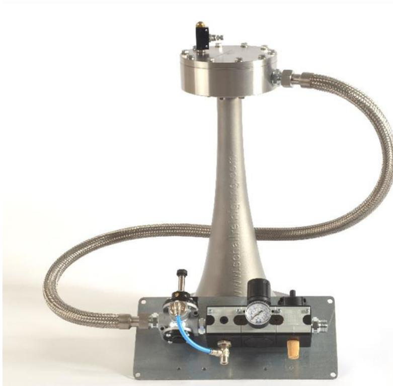
Our horns are manufactured by means of a precision casting process using stainless steel (1.4308 - standard alloy/ 1.4581/1.5415) or aluminium; generators and compressed air tubes are also made from stainless steel (1.4301). We use a special titanium steel alloy for the membranes and carbon for the seals.
